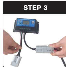
Then connect the controller onto the battery.
