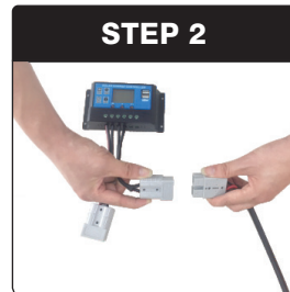
Disconnect the controller and battery.
